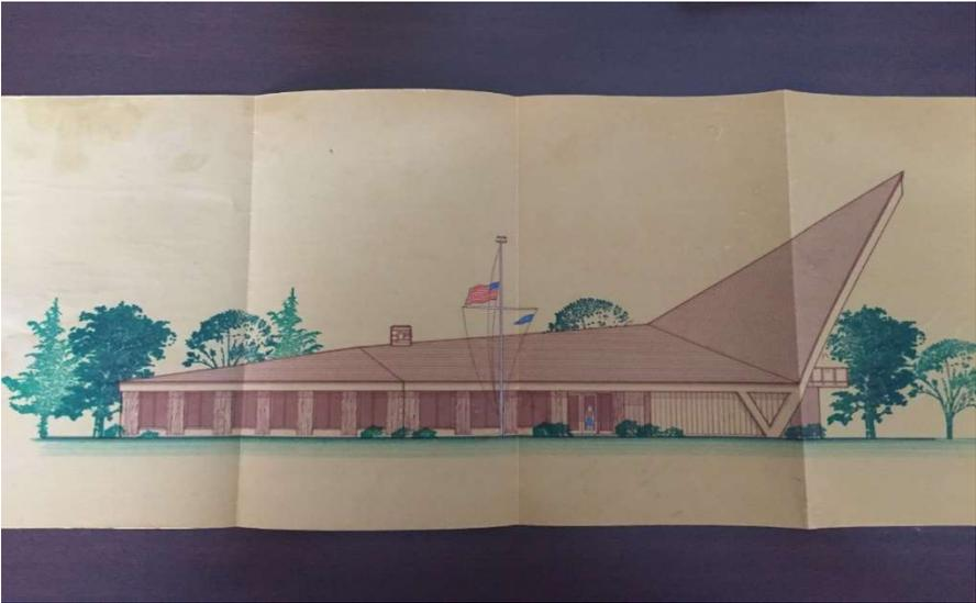
The exterior design of today's clubhouse is as originally drawn, but it was split into "first unit" and "second unit" for cost savings. The first unit was the spire and the structure surrounding it which would be built immediately, and the second unit which was the addition with sliding glass doors would be added later.
